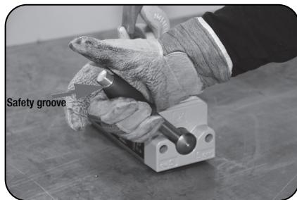
5. Make sure that the Lifting magnet is completely switched. As an indicator of this is true, the Safety groove on the gear lever, has to be completely visible
