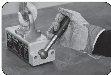
4. Turn on the lifting magnet at the workpiece (from right to left )
