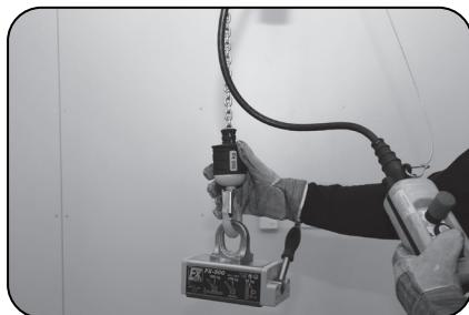
2. Move the lifting magnet with the crane on the workpiece slowly
