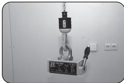
1. Attach the lifting magnet to a suitable for the lifting operation hoist so that it hangs horizontally
