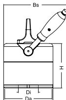
When transporting workpieces with different dimensions or properties, it must be ensured that a safety factor of 3 is achieved.
